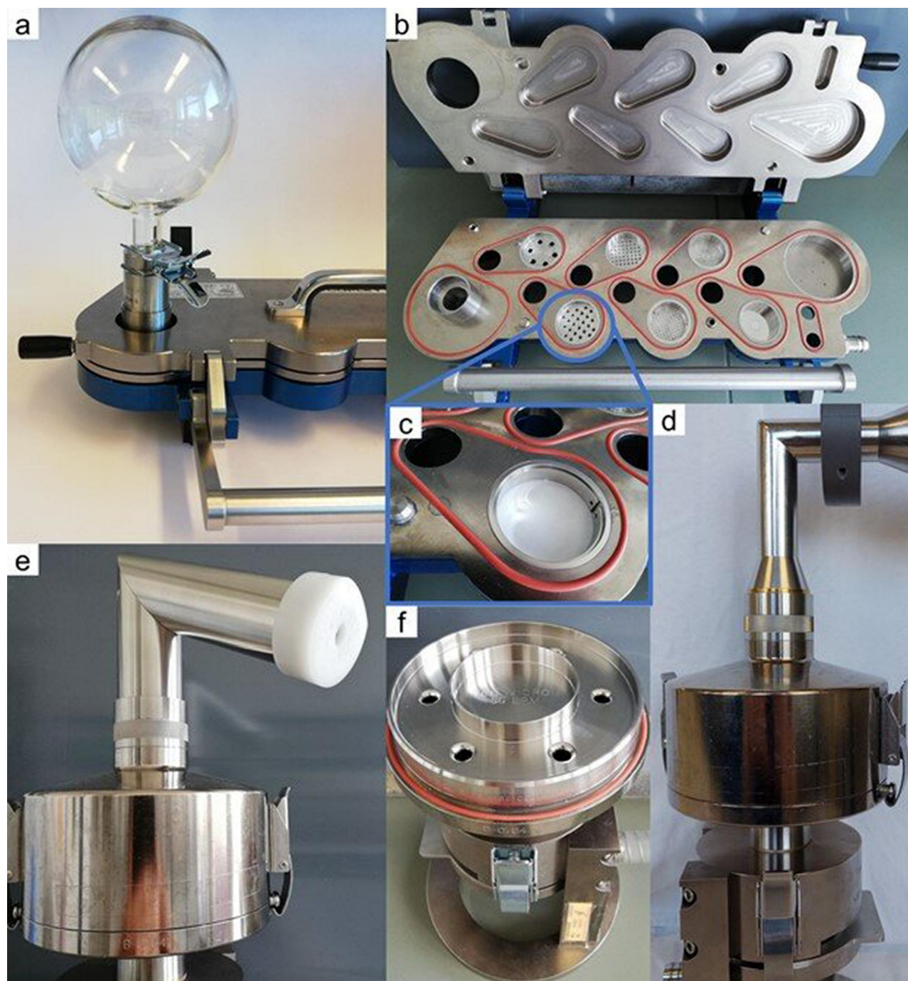
Figure 1. Commercially available impactors and inlets for aerodynamic assessment. The top half shows the Next Generation Pharmaceutical Impactor closed (a) and opened (b). (c) Illustrates the abbreviation of the NGI to the reduced NGI by inserting a filter holder and a filter into a selected nozzle of the NGI. The lower half shows the Fast Screening Impactor with a USP throat attached (d) and the metal induction port (e). Into the corpus of the FSI a 10 µm cut off plate at 30 L/min is inserted (f). A commercially available nasal inlet is the glass expansion chamber (a, 1 l variant shown).
