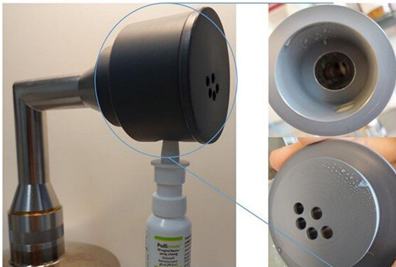
Figure 4. Left: KNI attached to the USP throat with a nasal spray inserted at the entry. Right: KNI after distribution of one spray shot (140 \mu\text{l} ) of Pollicom in the chamber. The aqueous solution deposits to the KNI ceiling.
