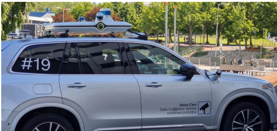
Figure 1.5: Presenting a data collection vehicle. The collected data is used for identifying relevant scenarios, utilized in the development of rule-based or machine learning software, and ultimately used for verification and validation.
