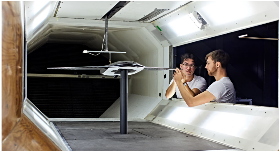
Figure 1 – Chalmers UAV platform mounted on a balance-arm in Chalmers wind tunnel
