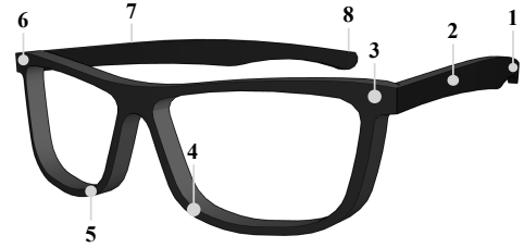
Fig. 1: Microphone positions on a pair of glasses as used in this study.
