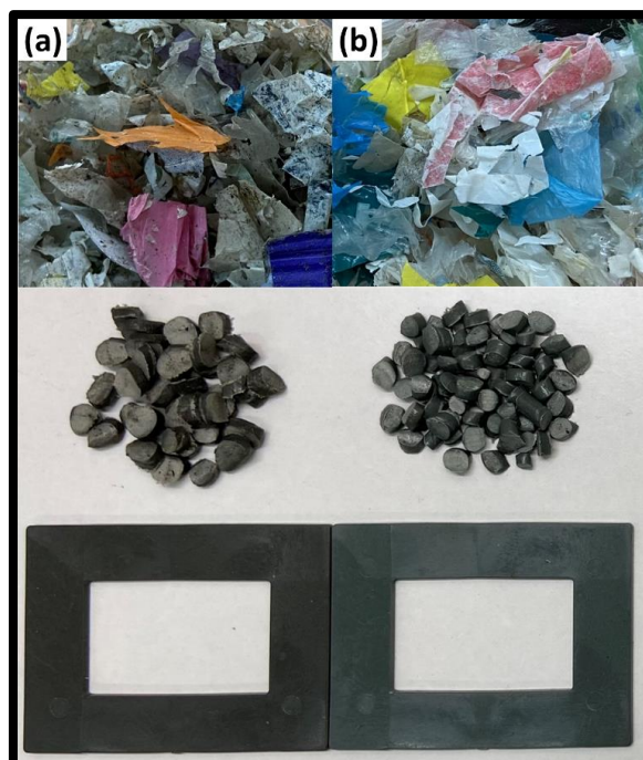
Figure 8. From top to bottom: the flakes, pellets and IM-sample of (a) the unwashed flexible PE material, (b) the laboratory-scale-washed flexible PE material.
