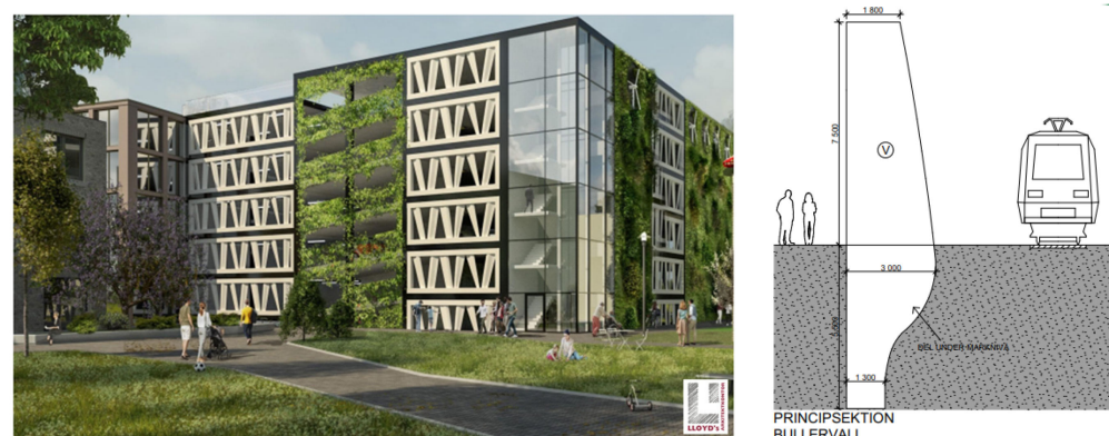
Figure 6. Case studies of EoS WTB repurposing in Sweden: façade elements for car park building (left) and noise barrier (right) (pictures from Lloyd's Arkitektkontor, Sweden).
