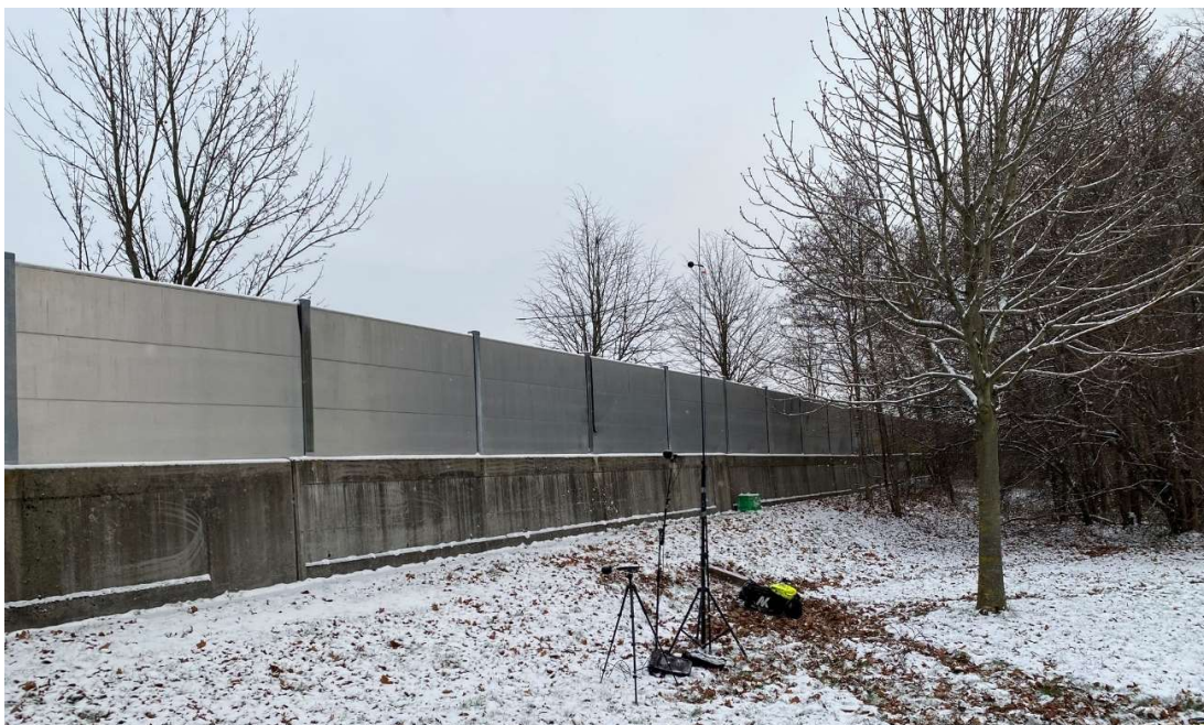
Figure 4.5: The measurement position 4 m behind the noise barrier at Site 2, south of the motorway (photo: Akustikkonsulten).
