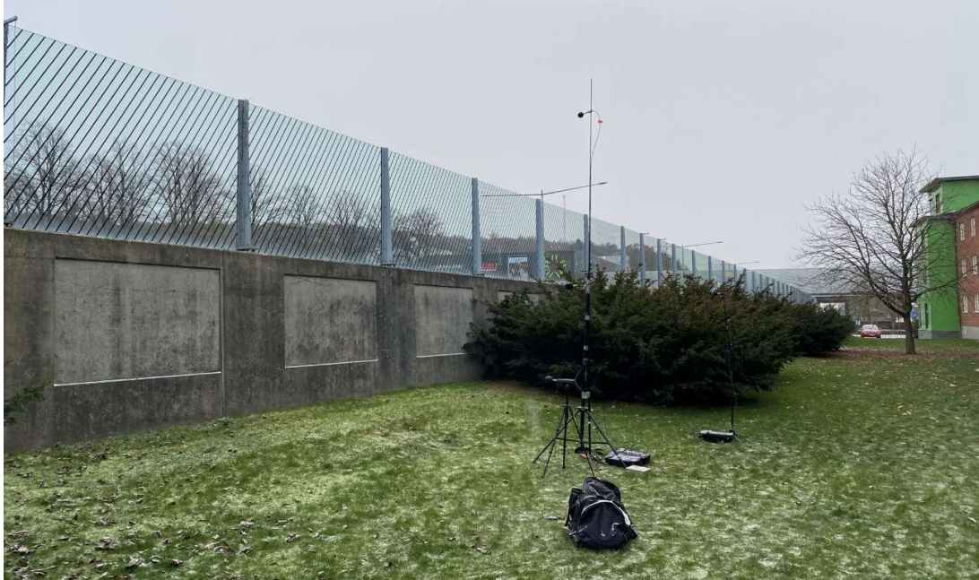
Figure 4.4: The measurement position 4 m behind the noise barrier at Site 1, north of the motorway (photo: Akustikkonsulten).
