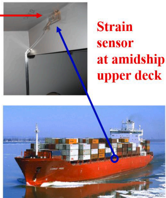
Fig. 6. The 2800TEU container ship utilized in this study, along with the arrangement of the strain sensor placement at the midsection, indicating the specific measurement point on the starboard upper deck.
