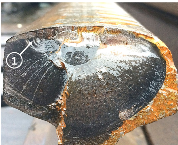
Fig. 8 Fractured rail with a shallow surface repair weld. Highlight 1 roughly indicates the surface repair weld [86]
