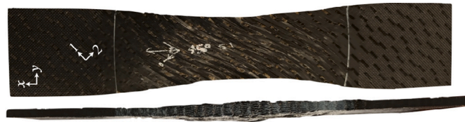
Fig. 13. Images of Sample 2 (45° off-axis loading) taken after the test showing necking, realignment of yarns and out-of-plane expansion.
