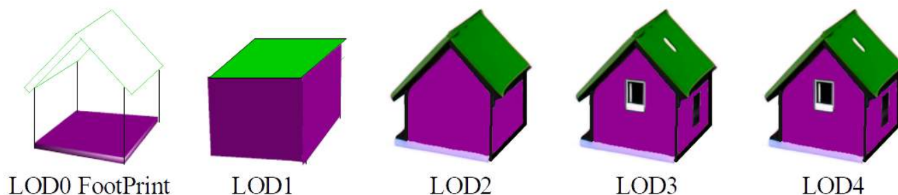
Figure 1. Different levels of detail (LODs) of building models according to Groger et al. [19].
