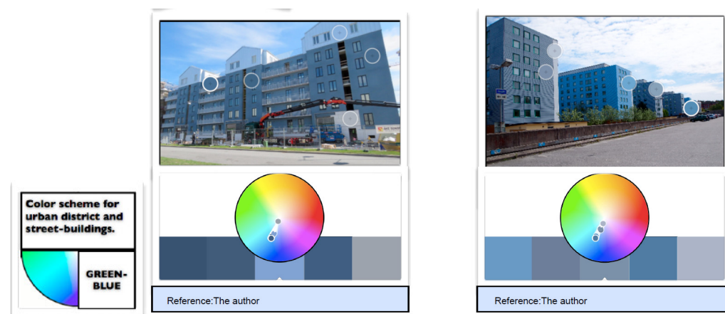
Scheme A3. The scheme shows a group of analogous colors located in the sector of the color wheel, which stretches from the green-blue color.
