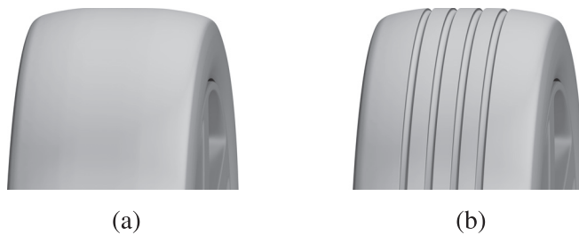
FIG. 3. Tread patterns considered for the DrivAer: (a) slick and (b) rain grooves.
