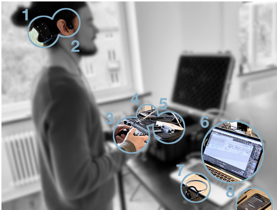
FIGURE 2. VR system, Parrot-VR, test setup: 1) IMU; 2) bone-conductive headphones; 3) controller; and 4) embedded computer. Auxiliary equipment: 5) audio interface; 6) laptop; 7) bone-conductive headphones; and 8) audio recording device. Note that the embedded computer hosts the software of both Parrot-VR and the Audomni ETA. Figure and caption originally produced for this work, but published first with slight differences in [27].
