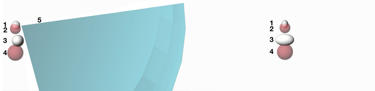
FIGURE 4. VR avatar in default positioning, from the side and front. White spheres are head (1) and body (3), and red their pivot points (2 and 4), blue cone (5) is the sensor FoV (omitted on the right). The body can affect the sound feedback by occluding the FoV, which happens for many possible head rotations. All sizes and relative positions that might affect this are based on a hypothetical female user with relevant features at the, in this regard, most disadvantageous 95th percentile of anthropometric data. The avatar model determines sensor placement, pivot points, and acts as a possible occluding agent for the sensor FoV, but not collisions. Collisions are instead determined by if the horizontal distance between the body pivot point and a collision object is too close, regardless of its height. Note that, since lower torso and extremities are thus both unnecessary for collision detection and redundant for sensor occlusion, they are omitted from the model. Figure and caption originally produced for this work, but published first with slight differences in [27].
