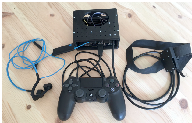
FIGURE 1. VR system, Parrot-VR, system hardware. Clockwise from left: bone-conductive headphones; embedded computer and audio interface; headband with IMU; controller. Figure and caption originally produced for this work, but published first with slight differences in [27].
