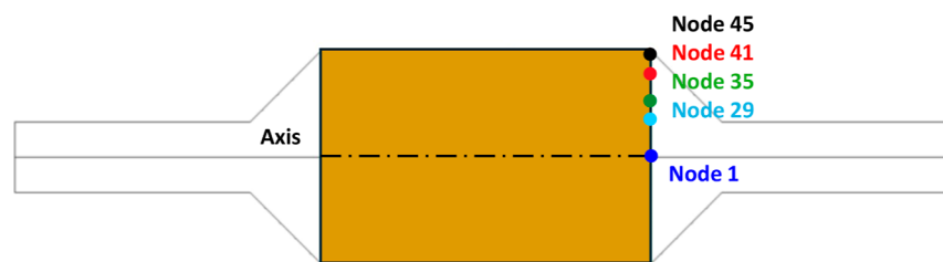
Figure 9. Node locations chosen by D-optimal design. Nodes 1, 29, 35, 41, and 45 are chosen. Three of the five chosen nodes are located closer to the wall.
