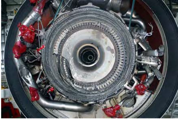
Figure 1.1: Rear face of the broken stage-1 HPT disk from a Boeing 767-219ER (General Electric CF6-80A high-bypass turbofan engine). The fracture originated on the left side of the disk, the initial part of the crack broke intergranularly. Figure reprinted with permission from ATSB air safety investigation report 200205780 [2].
