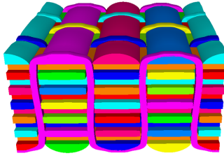
Figure 4.1: SVE of a 3D fibre composite generated by Texgen.
