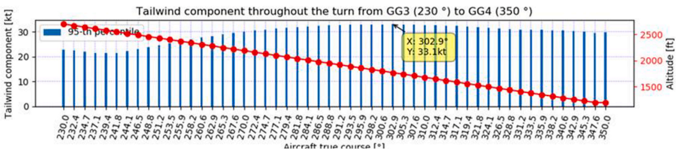
Fig. 5. The calculated TWC assuming a 3° descent angle throughout the fictitious turn from point GG3 to GG4 @ESGG.
