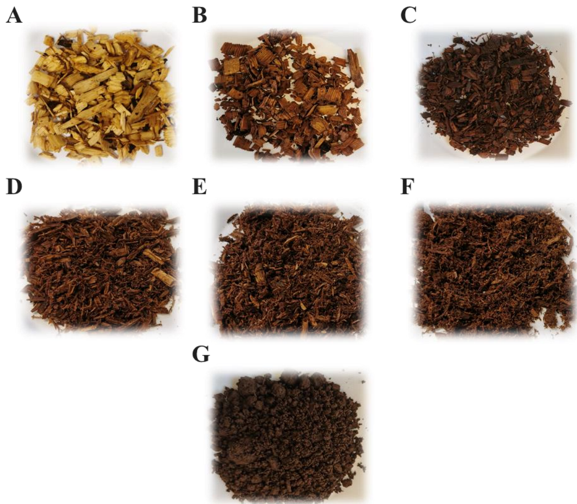
Figure 3.2. Images of the different pretreated materials. (A) raw material, (B) STEX 180°C /auto, (C) STEX 210°C /auto, (D) STEX 210°C /HAc, (E) STEX 210°C /H 3 PO 4 , (F) STEX 210°C /H 2 SO 4 , and (G) STEX 210°C /SO 2 .
