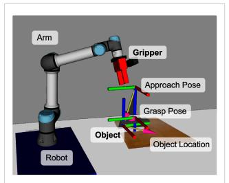
Robot using a pick skill with a visualization of the necessary parameters. To run this skill, we only need the Gripper and the Object parameters. SkiROS2 can deduce all other necessary parameters through a set of rules in the skill description shown in listings 4 and 6.
