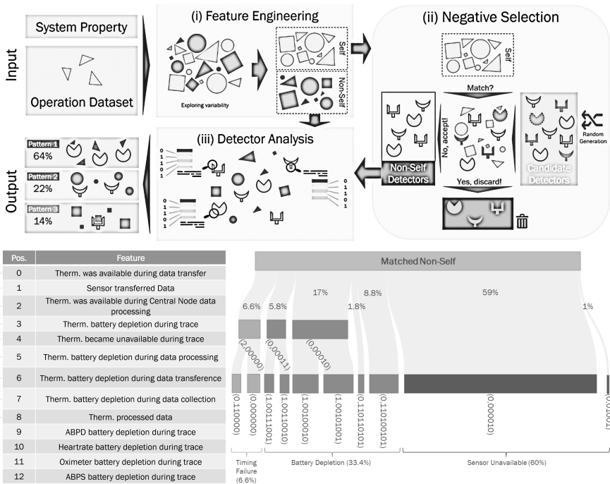
Figure 3.6: Overview of the pipeline to automated explanation using the negative selection algorithm. Note: originals in Chapter 9
