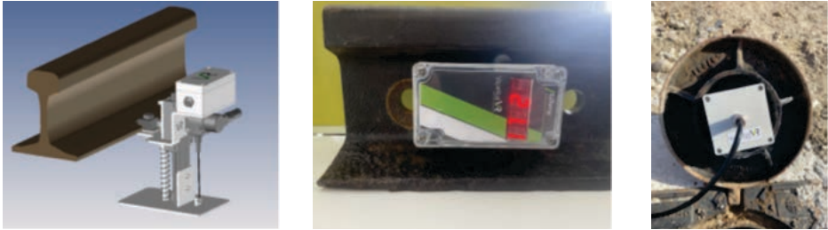
Figure 23-1 Examples of sensor node integration: (a) Acceleration sensor, (b) Temperature sensor, (c) Water level sensor
