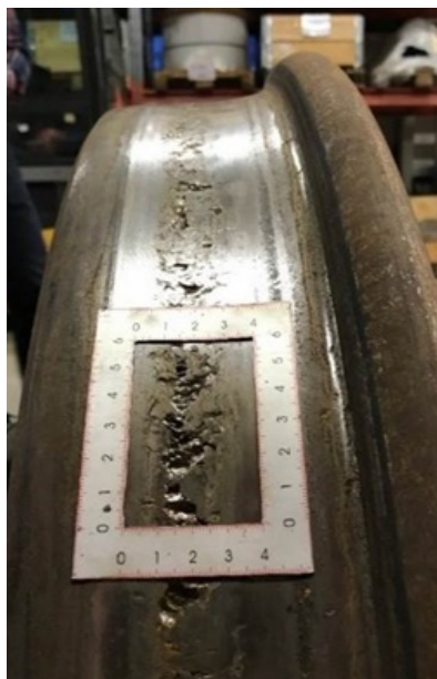
Figure 44-1 Wheel with severe rolling contact fatigue damage
