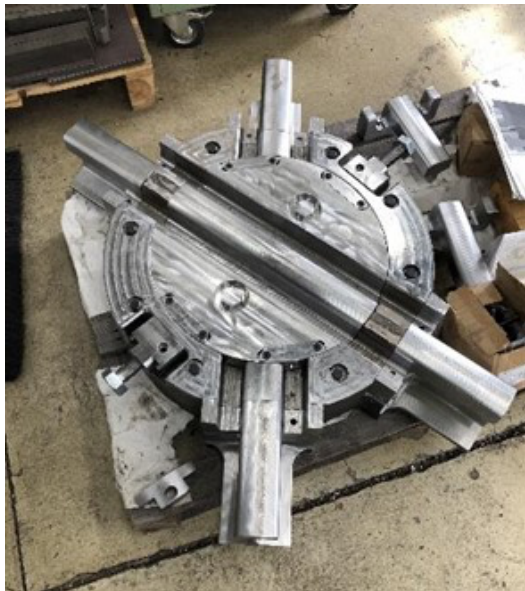
Figure 10-1 First build-up Concentric Moveable Crossing
