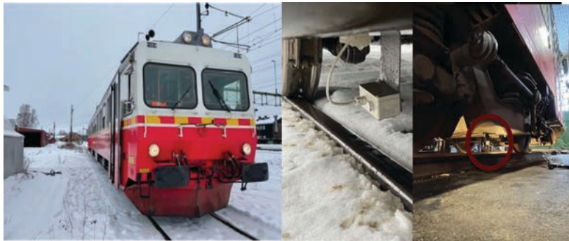
Figure 72-1 Mounting of friction level sensor on train.
