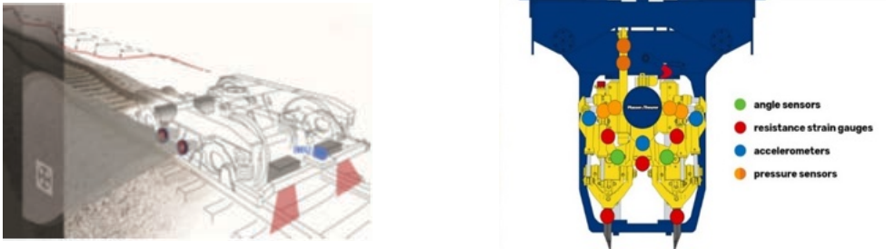
Figure 78-1 A representation of the ATG system: Marker, stereo cameras, IMU and laser sensors (left). The tamping unit (TAMP) with the sensors equipped (right)
