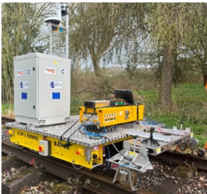
Figure 20-1 Autonomous rail inspection trolley
