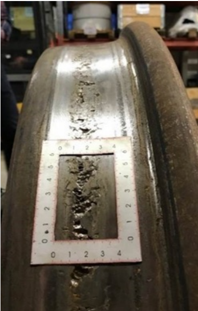
Figure 44-1 Wheel with severe rolling contact fatigue damage
