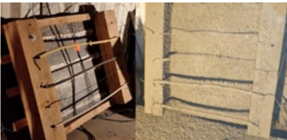
Figure 55-1 Resistance test support – before / after
