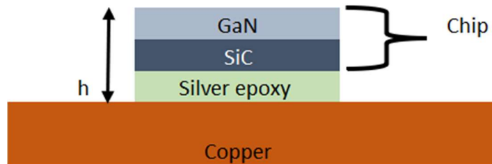
Figure 5. GaN chip mounted on copper carrier using a silver epoxy TIM [Paper A]
