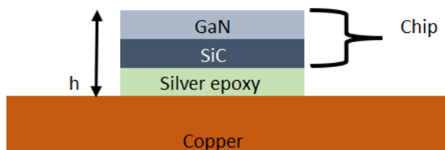
Fig. 1. Cross section of bare die on copper, not to scale.
