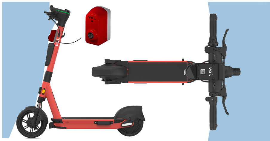
Fig. 2. Camera mounted on the e-scooter and visualization of the camera's field-of-view (area colored in blue). (For interpretation of the references to colour in this figure legend, the reader is referred to the web version of this article.)
