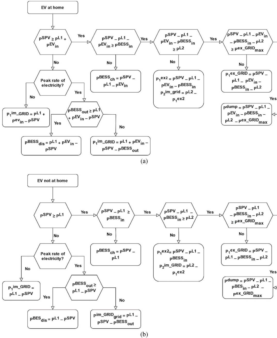
Fig. 2. Flow chart for the rule-based home EMS: energy sharing between home-1 and home-2 when: (a) EV is at home-1; (b) EV is not at home-1.
