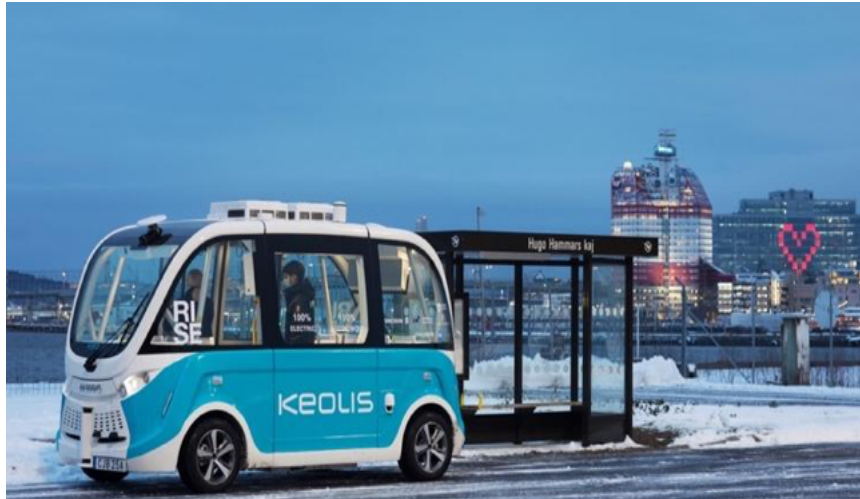
Figure 10 The Navya Arma used in the Gothenburg pilots, accommodating approximately 12 persons in the vehicle. Permissions for photo granted by RISE.
