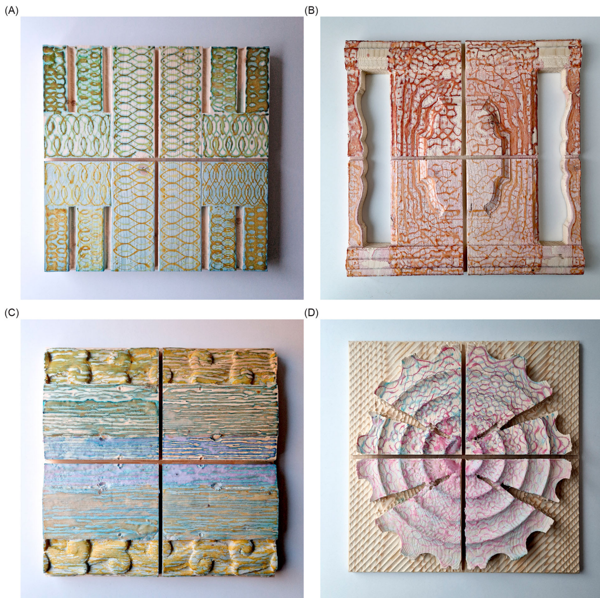
Figure 7. Architectural features of biobased coatings at the macroscale, with final appearances resembling the initial digital pattern designs. (A) The ichthys pattern discernible on the wall cladding fragment. (B) The Voronoi pattern discernible on the mezzanine railing fragment. (C) The flowline pattern discernible on the frieze fragment. (D) The circular pattern discernible on the sculpted beam fragment.
