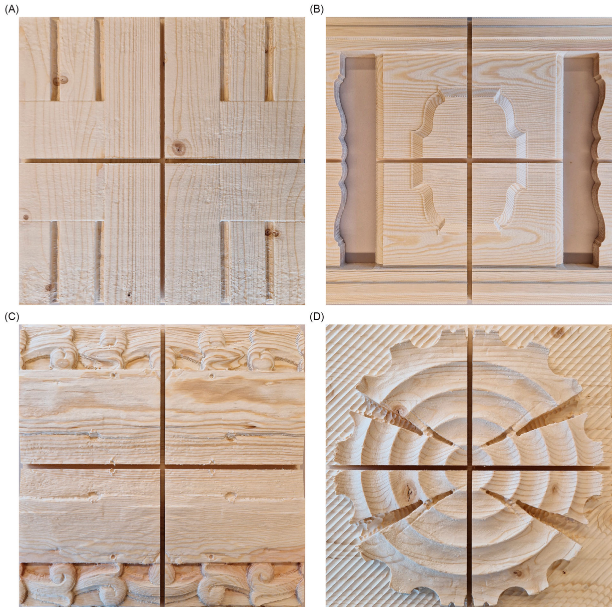
Figure 3. CNC-milled mockups of architectural detail fragments sampled from existing sites. (A) Wall cladding fragment. (B) Mezzanine railing fragment. (C) Frieze fragment. (D) Sculpted beam fragment.
