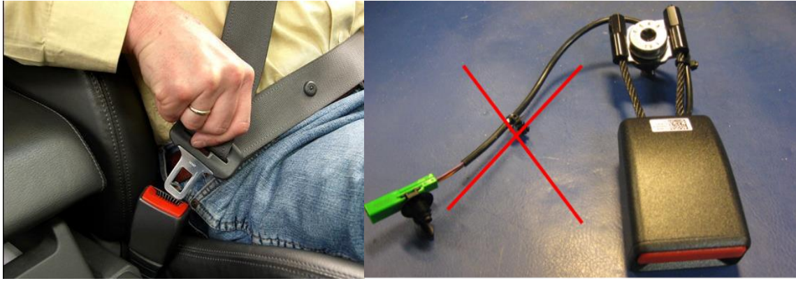
Figure 16. Belt buckle including cable harness and connector.
