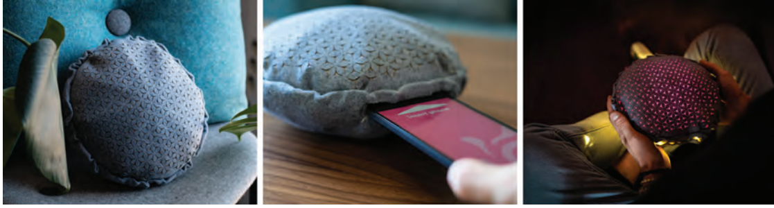
Figure 1.1: Azalea: idle (left), initialised by “swallowing” the phone (center), in use by animating the pillow with the phones actuators (right).
