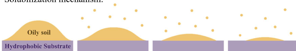
Figure 5. Mechanism of liquid soil removal from surfaces. In the roll-back or roll-up process, surfactants from the cleaning solution penetrate the crevices between the soil and substrate, increasing the contact angle of the liquid soil with the surface and creating an osmotic flow that aids in detachment. For hydrophobic substrates, however, soil removal relies on lowering the oil-water interfacial tension, allowing the surfactant to either solubilize or disperse the soil through micellar solubilization or emulsification.
