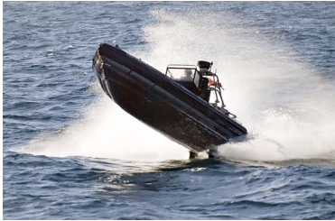
Figure 1: A fast RIB (rigid inflatable boat) exposed to a severe acceleration environment [https://commons.wikimedia.org/wiki/File:RDN_RHIB.jpg].
