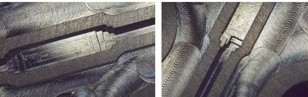
Fig. 4. Photos of the block with back-to-back twists. The block manufactured from aluminum alloy. Waveguide dimensions are 380 x 760 \mu\text{m} .
