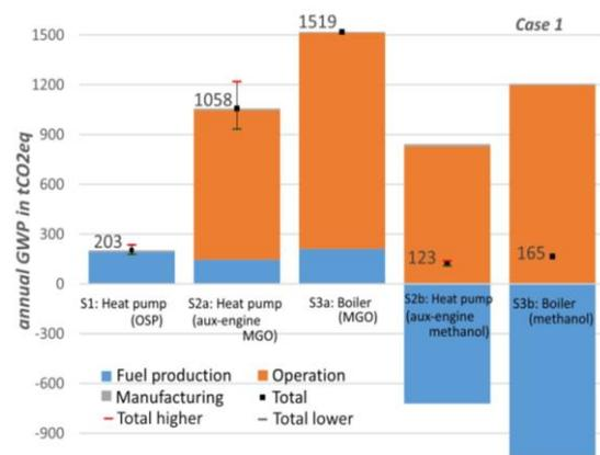
Figure 3: GWP of different scenarios for the first case study vessel. Total higher is total GHG emission considering heat pump COP 3 and lower is for COP 4.
