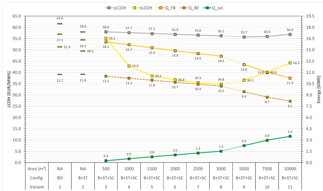
Fig. 6. Energy use and heat cost 1 – overview of energy use and resulting LCOH for variant 1 and 3 – 11 simulated in this study. Beware the non-linear x-axis in the figure.
