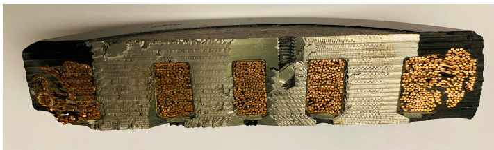
Figure 3.9: AFM-2 semi enclosed slots
