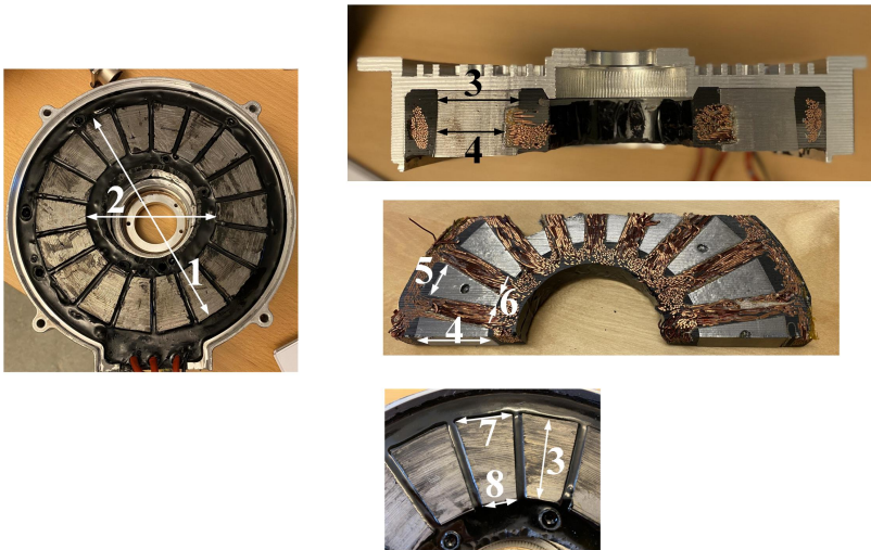
Figure 3.7: Radial measurement - Stator of AFM-2. 1 - Outer diameter of the stator; 2 - Inner diameter of the stator; 3 - Length of the tooth; 4 - Tooth body width at the cutting surface, when the stator cutting is along the white dashed line, seen in Figure 3.6; 5 - Tooth body outer width; 6 - Tooth body inner width; 7 - Tooth tip outer width; 8 - Tooth tip inner width
