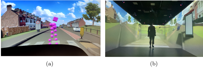
Figure 2.3: Illustration for the distributed simulator study. (a) A pedestrian from the driver's view: the pink spheres represent body markers attached to the pedestrian. (b) An interaction example from the third view: a pedestrian is at the zebra crossing and interacting with the vehicle to their right.
