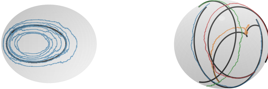
FIGURE 1. Left: Trajectories of components of the angular velocity in the rigid body equations. The lines show numerical solutions to the deterministic equations (black) and the stochastic equations (blue). Note that both trajectories remain on the unit sphere, depicted in gray. Right: Trajectories of four point vortices on the sphere, following the deterministic dynamics (black) and stochastic dynamics (colored).
