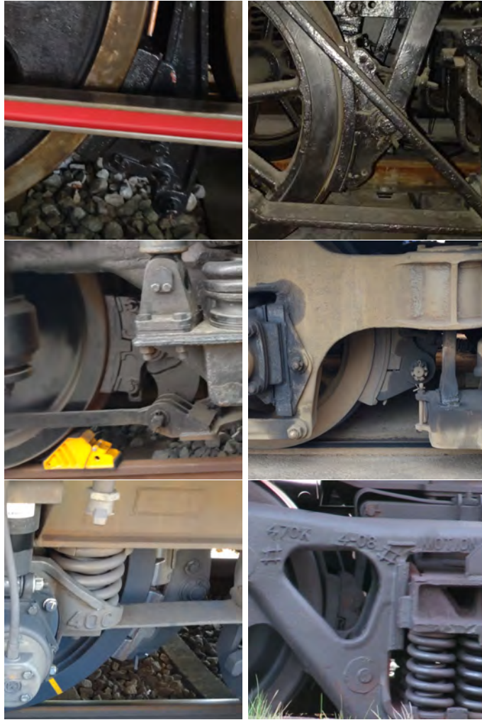
Figure 2.4: Brakes blocks used on different trains in different eras. From upper left, row by row: 1) Japanese C62 steam locomotive, 2) Japanese KuMoHa 40 passenger car, 3) EF81 electric locomotive used on 'Twilight Express' services in Japan, 4) Series 7000 tram used in Hakodate city, 5) SJ B10 passenger car in use on the Stockholm-Uppsala commuter line 6) Fammoorr type 050 freight wagon as used on the Swedish-Norwegian Iron ore line.
