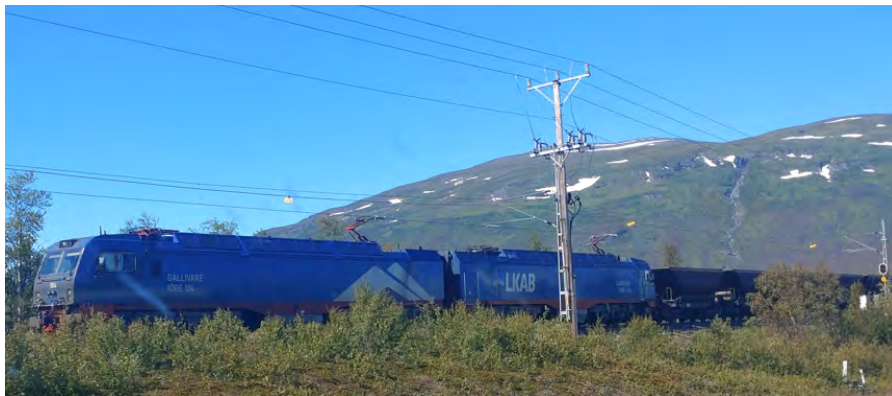
Figure 1.2: LKAB Iron ore train on the Swedish iron ore line. This is currently the most heavily laden train line in Europe with regards to axle load, with an axle load limit of 31,5 tons. As with most freight cars, the iron ore wagons are equipped with tread brakes.
