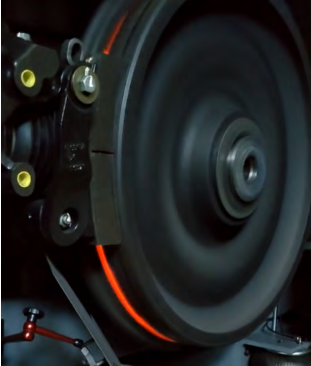
Figure 3.1: Wheel during drag braking applications, where the high tread temperatures in the brake contact strip cause the steel to glow.
