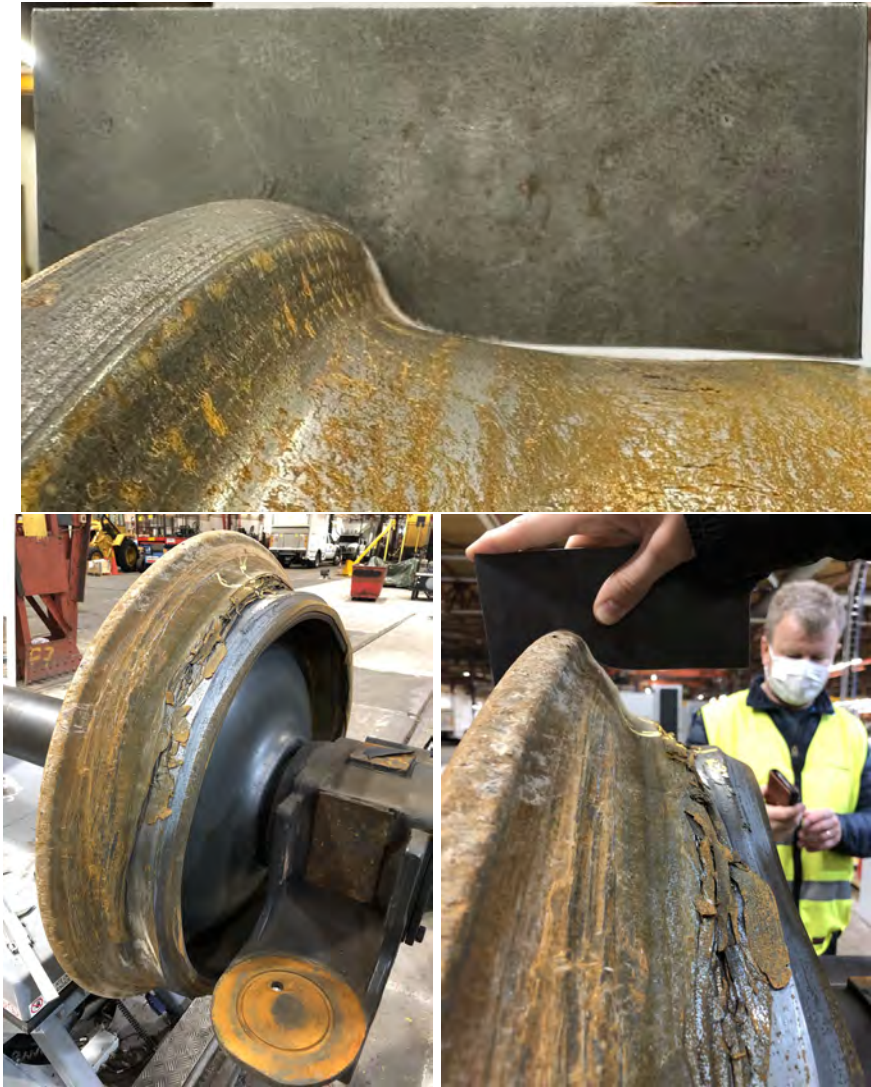
Figure 4.5: (Above) Hollow wear on a railway wheel, showing the difference at both tread and flange compared to nominal profile. Picture courtesy of Henrik Nordin, Lucchini Sweden. (Below) Thermal overload causing (significant) plastic deformation and material flow on a railway wheel.
