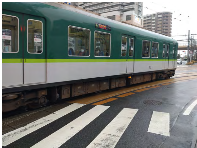
Figure 1.3: Keihan 800 series electric multiple unit (EMU) commuter train in Biwako-Hamaōtsu, Kyoto, Japan. This specific model, in use on the Keihan Keishin-line, is designed for mountain railways due to the gradient between Kyoto city and Biwako-Hamaōtsu. It is the only Japanese example of a commuter train with cast iron brake blocks.
