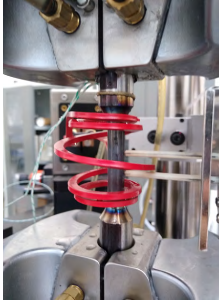
Figure 6.2: MTS 809 test frame with ER7 wheel steel specimen and induction coil.
