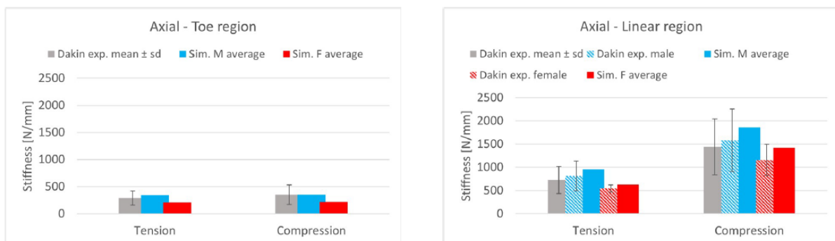
Figure 33. The resulting PS joint stiffness in tension and compression. From (Brynskog et al., 2022).
