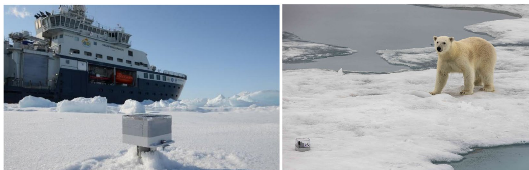
Fig. 3 Left: illustration of the OMB deployment on top of a frozen-in mount to elevate the box over the sea ice. Picture taken in the context of the CIRFA_UIT deployment, credits Johannes Lohse, UiT, reproduced from 54 . Right: illustration of the OMB deployment directly on the sea ice. Picture taken in the context of the AWI_UTOKYO deployment, credits Mario Hoppmann.
