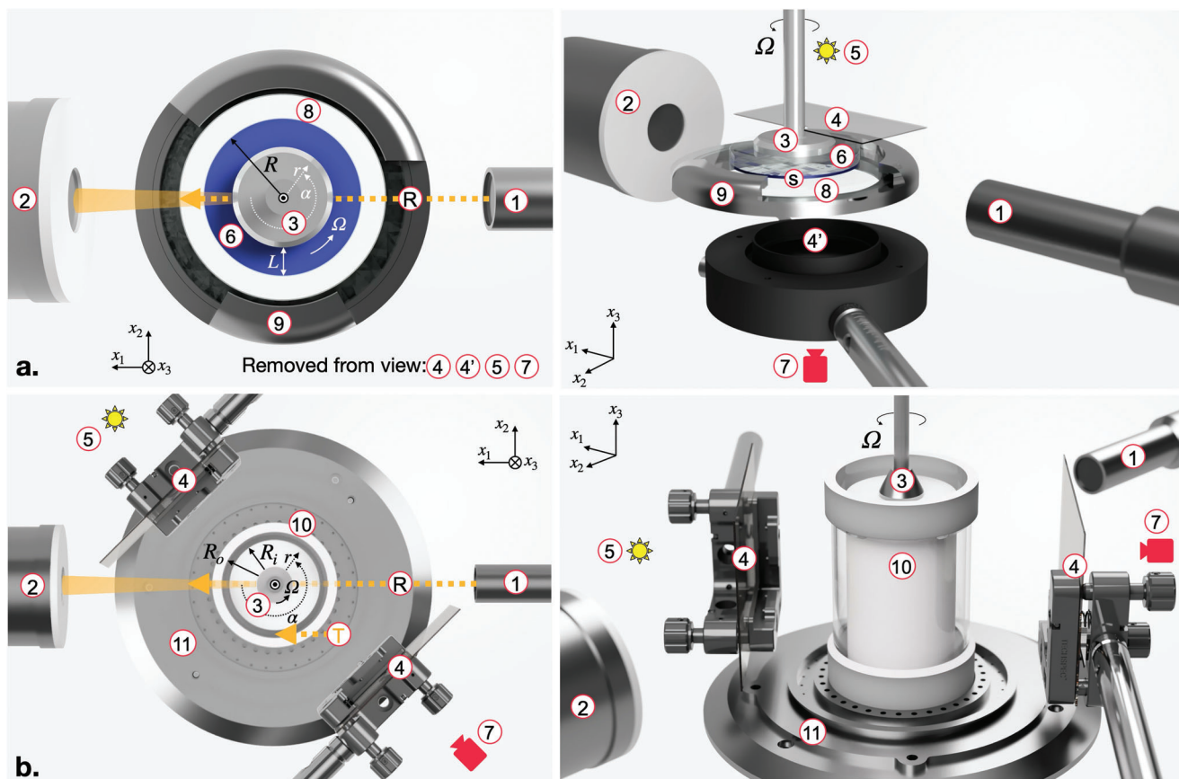
Figure 5. Schematic of the Rheo-PLI-SAXS custom experimental setups: a) using a parallel-plate and b) a concentric-cylinders measuring geometries. Notations: (R) – radial incident X-rays, (T) – tangential incident X-rays, (1) – X-ray source, (2) – detector tube, (3) – steel part of the measuring geometries (4,4') – polarizer / analyzer, (5) – LED light source, (6) – transparent part of the upper plate measurement geometry, (7) – DSLR camera, (8) – glass bottom plate, (9) – custom bottom plate holder, (10) – outer cylinder, (11) – concentric cylinder setup mounting system; (s) – sample (not included in the bottom row to preserve clarity).
