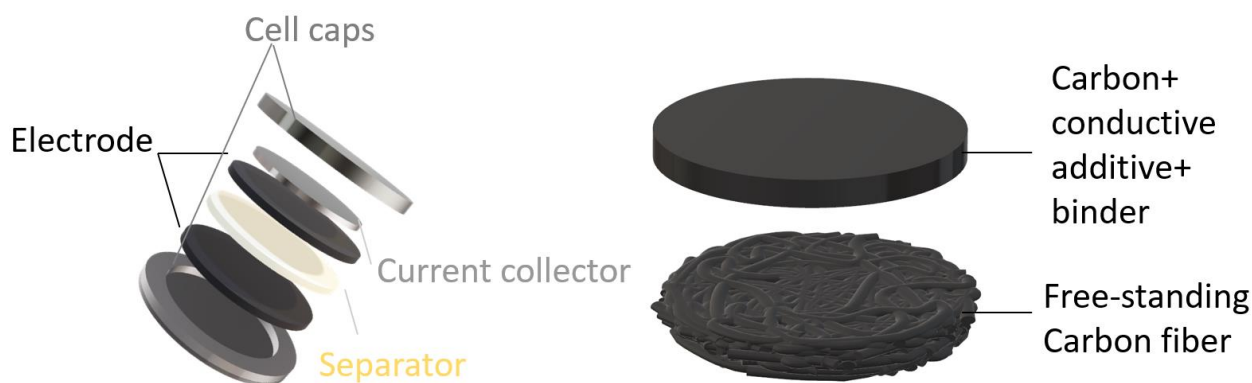
Figure 14. Schematic representation of a coin cell and its different components with some of their different electrode forms.
