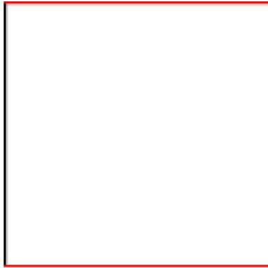
**Fig. 9** For a rectangular domain we impose the Dirichlet boundary condition on the red sides and Neumann boundary condition on the black sides
