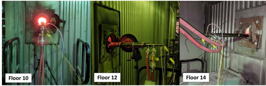
Fig. 1 Images of University of Utah narrow-angle radiometer setup at each boiler elevation examined
