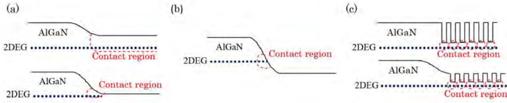
Fig. 3.3. (a) shallow recessed contacts and a trade-off between etching depth and 2DEG density, (b) deeply recessed contacts, and (c) patterned recessed contacts [5].
