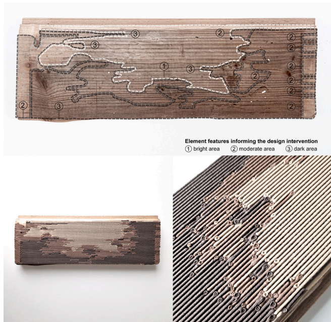
Fig. 12. Design outcome of experiment four, embracing reclaimed wooden floorboard (top) with new coating that approximates, through coloring variations, discolorations of piece underneath (bottom left and right). Texture generated using parametric construction methods informed by color data registered for treated piece via robot vision and extracted using 3D point cloud data filtering.
