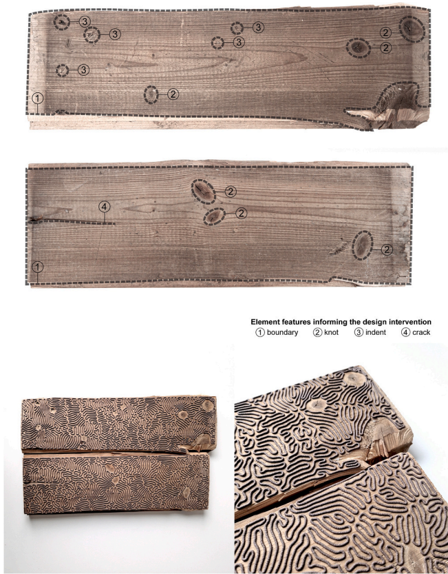
Fig. 6. Design outcome of experiment one, embracing two reclaimed wooden floorboards (top) decorated with new 3D printed textures (bottom left and right) generated using differential growth algorithm adapting to unique shapes and layouts of wood knots, cracks, and irregular outlines of treated pieces, found using ML.
