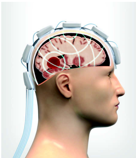
Figure 1.5: A generic sketch of a microwave-based stroke diagnosis system [18]
