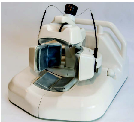
Figure 1.6: The Strokefinder device, MD100, developed by Medfield Diagnostics AB [36], [43]
