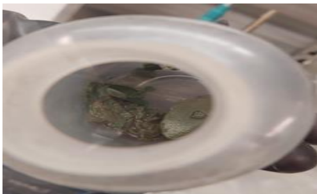
Figure 5. Coprecipitated solid of U and Ce ( \text{Ce}_{0.10}\text{U}_{0.90} ) after centrifugation and removal of supernatant.
