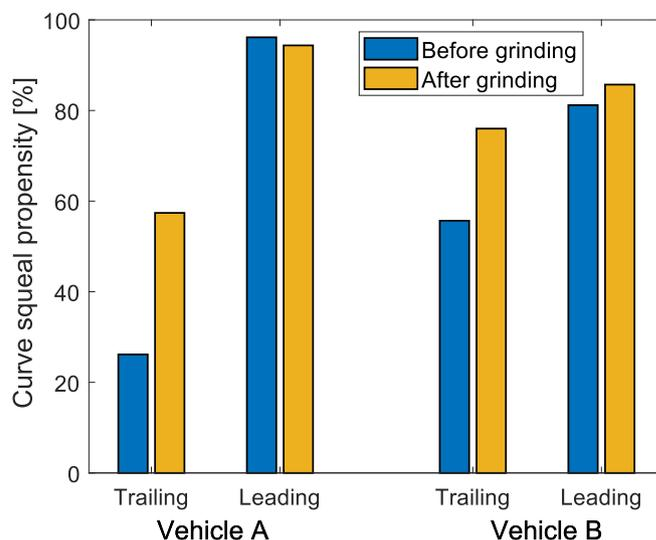
Fig. 5. Comparison of inner wheel squeal propensity for both vehicles evaluated for vehicle passages performed before and after rail grinding, separately.
