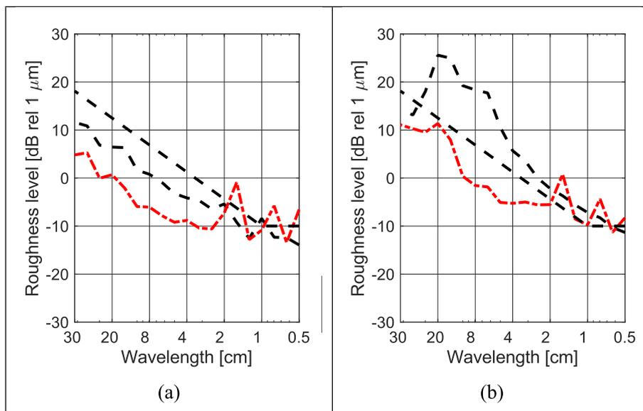
Fig. 2. Roughness level spectra in 1/3 octave bands based on measurements before and after rail grinding of the high (a) and low (b) rail on the studied curve. Roughness levels are averaged from measurements in three parallel lines over a distance of approximately 100 m. - - -: Before rail grinding, - - -: After rail grinding, —: Limit according to ISO 3095.
