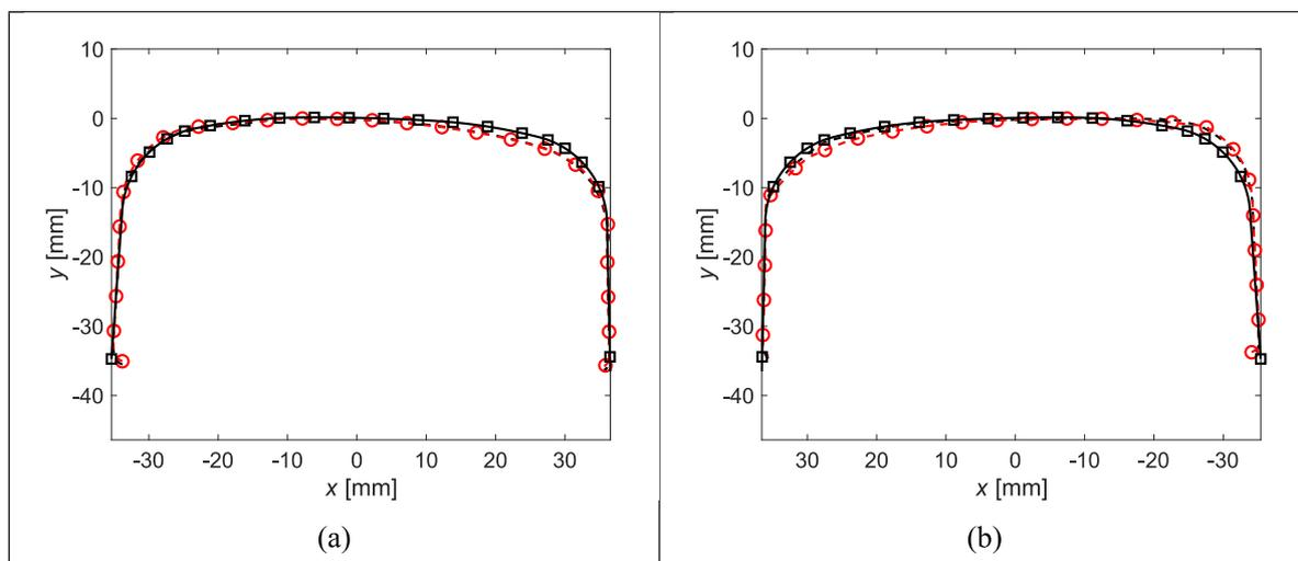
Fig. 1. Rail profiles measured at the high (a) and low (b) rail before (---) and after (-○-) rail grinding on the studied curve. —□—: Nominal BV50 rail profile with inclination 1:40.
