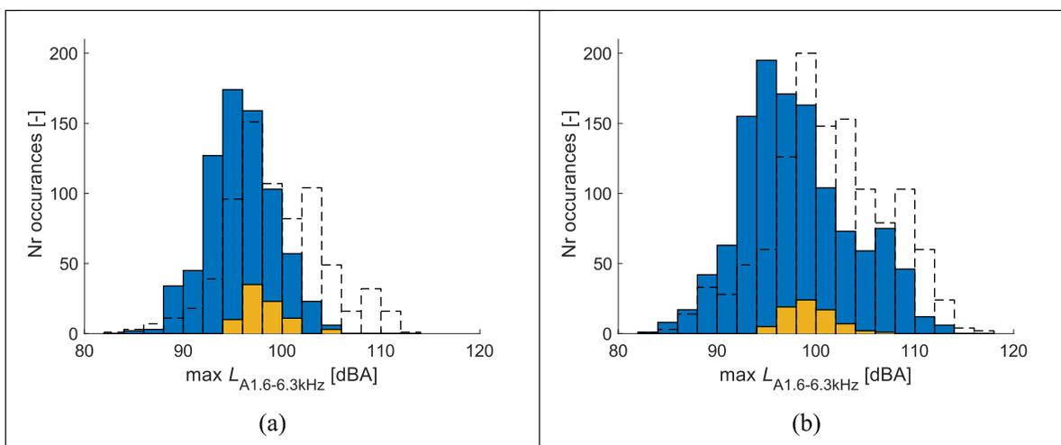
Fig. 7. Histogram of maximum A-weighted and passband filtered (between 1.6–6.3 kHz) sound pressure levels recorded in the studied 213 m radius curve by the QTMS-system mounted on vehicle A (a) and B (b) during one year of regular traffic. ■: Outer wheel and no detected squeal, ■: Outer wheel and detected squeal, - - -: Inner wheel.
