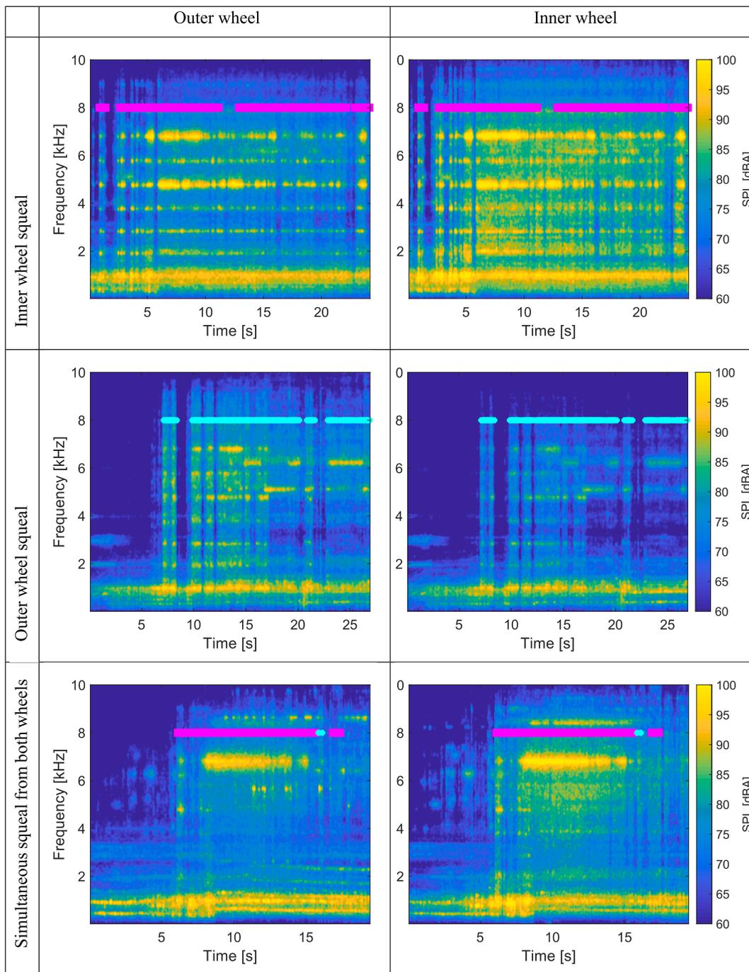
**Fig. 8.** A-weighted sound pressure level spectrograms obtained from the microphones belonging to the QTMS-system mounted close to the inner (right column) and outer (left column) wheel–rail contacts, respectively. Examples of passages that are characterized by squeal emitted from the inner wheel (top row), outer wheel (middle row) and simultaneous generation from both wheels (bottom row). ■: Inner wheel squeal detection, ■: Outer wheel squeal detection.
