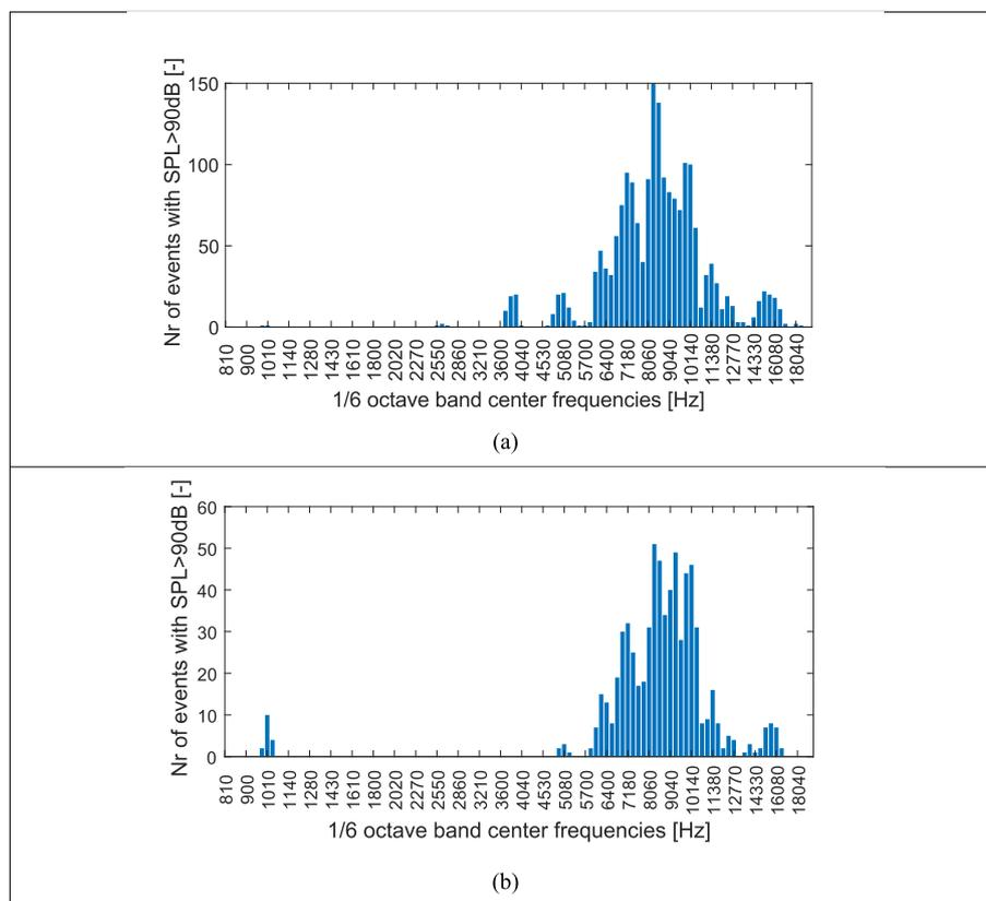
Fig. 4. Histogram of squeal events identified as spectral components with sound pressure level exceeding 90 dB. The analysis is based on 1/24 octave band spectrum evaluated for windows of 1 s length. The results of (a) and (b) are obtained from wayside noise measurements of 69 vehicle passages performed at locations separated by 50 m in the studied circular curve of 213 m radius.
