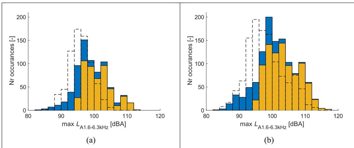
Fig. 6. Histogram of maximum A-weighted and passband filtered (between 1.6–6.3 kHz) sound pressure levels recorded in the studied 213 m radius curve by the QTMS-system mounted on vehicle A (a) and B (b) during one year of regular traffic. ■: Inner wheel and no detected squeal, ■: Inner wheel and detected squeal, - - -: Outer wheel.
