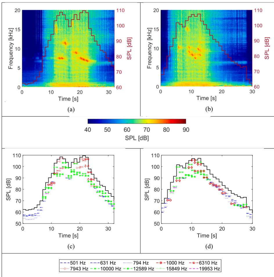
Fig. 3. (a) and (b): Examples of sound pressure level (SPL) spectrograms measured during pass-by of two vehicles. The solid line shows total SPL evaluated for window length 1 s and taking into account the frequency range above 400 Hz. (c) and (d): The three 1/3-octave bands with largest SPL together with the total SPL evaluated for windows of 1 s length. Results in sub-figures (c) and (d) corresponds to passages (a) and (b), respectively.
