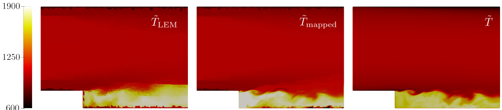
Figure 4.3: Instantaneous temperature: LEM-level \tilde{T}_{\text{LEM}} (secondary output), LES resolved \tilde{T} (iterated from \tilde{h} ), and LES resolved \tilde{T}_{\text{mapped}} (from mapping closure).
